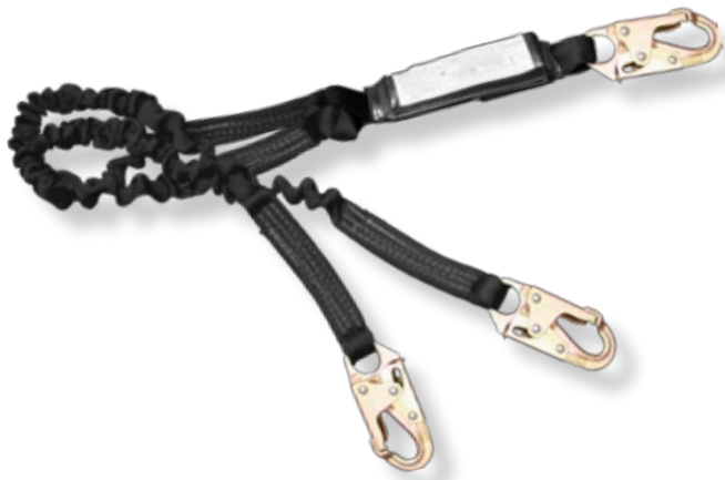
22440AS 6' 100% tie-off pack style shock absorbing lanyard 1 3/8" wide tubular webbing Relaxed length of 4 1/2' Z74 locking snaphooks each end
