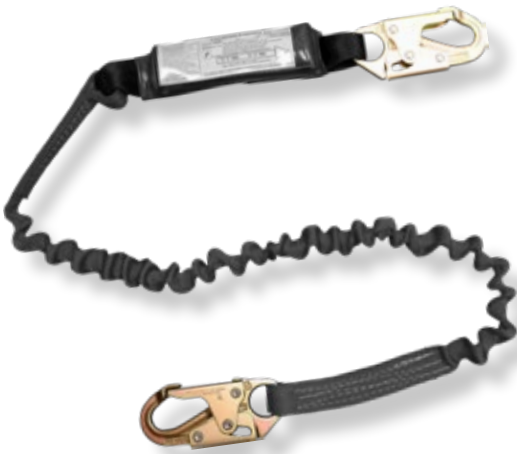
22450AS 6' pack style shock absorbing lanyard 1 3/8" wide tubular webbing Relaxed length of 4 1/2' Z74 locking snaphooks each end
