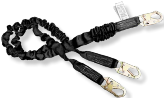
22420AS 6' 100% tie-off tubular style shock absorbing lanyard 2" wide tubular webbing Relaxed length of 4 1/2' Z74 locking snaphooks each end
