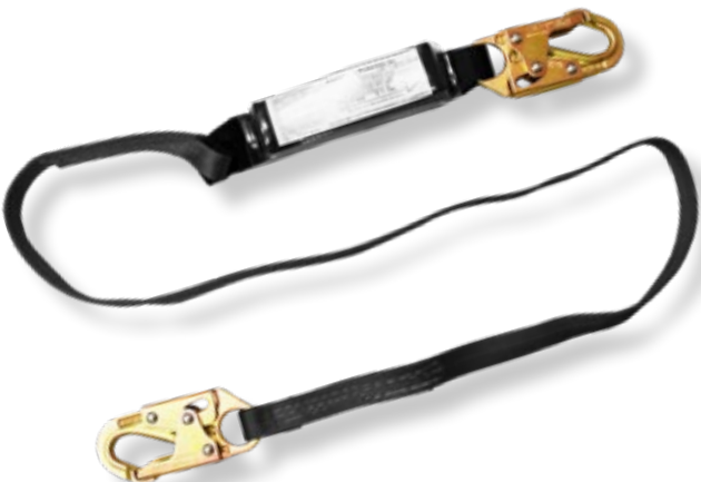
22450A 6' pack style shock absorbing lanyard 1" wide webbing Z74 locking snaphooks each end
